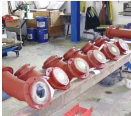
The material ABRESIST/KALCOR is used to line steel pipes
