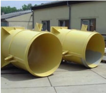
Mixer silos are lined with the material KERAFLEX
