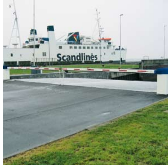
Solution combining two opposing large barriers for lorry entrance to a seaport
