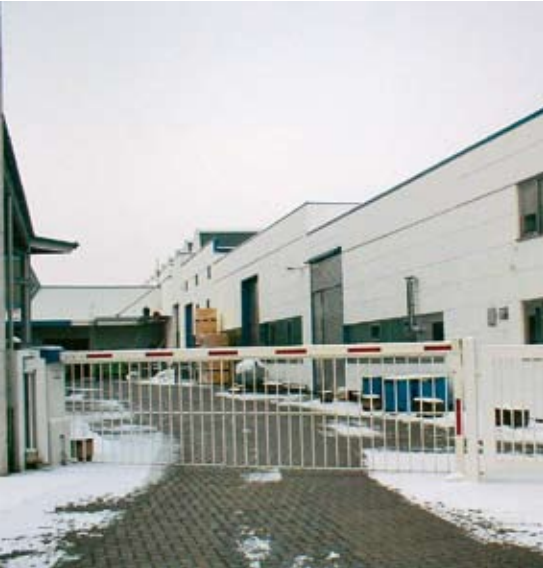
Special road barrier with enhanced height, hanging grid and housing mounted on a pedestal and separated pedestrian access
